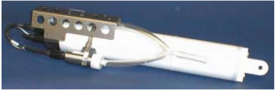
SBE 19plus SEACAT with SBE 5M pump
