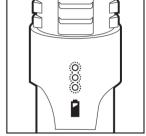
To set the laser to full-power/momentary mode, hold the SmartSwitch and press the tailcap button. After unlocking the laser, the 3 LEDs will be lit up.
