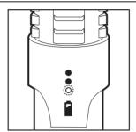
To unlock the laser you only need to **push** the SmartSwitch quickly three times and then hold it for less than 1 sec. two times.
