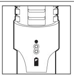
To switch to **medium-power mode**, you may hold the SmartSwitch button until the 2nd LED lights up.
