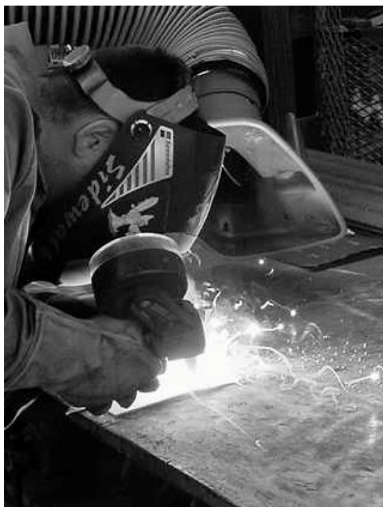
Welding Fumes Extraction
