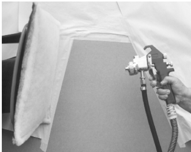
Spraying Toward Filter Hoods
