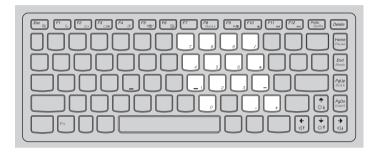
**Note:** The Num lock indicator will light on if the numeric keypad is enabled.
