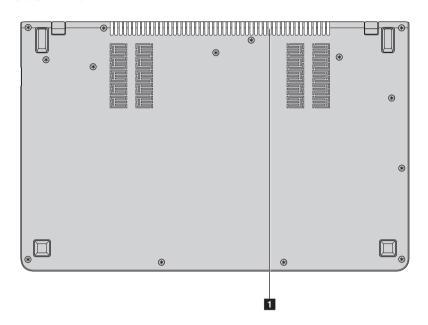
**1 Fan louvers** Dissipate internal heat.
