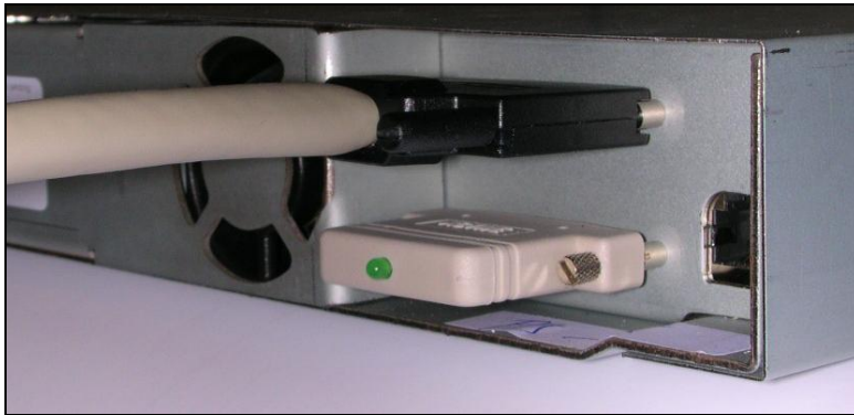
Figure 11. SCSI cable and SCSI terminator connection
