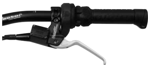
Brake lever (master cylinder) MAGURA Gustav M
