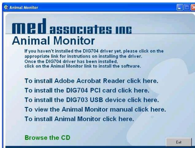
From the screen shown in Figure 1.1, select the type of DIG-704 device being used, and then follow the instructions to install the device drivers. Once all of the necessary drivers have been installed, select **To install Animal Monitor click here.**
