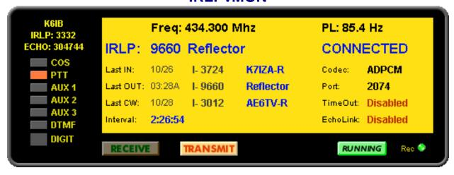
The IRLPvMON Monitor Screen is a display that shows the real-time status of the node. It is a Monitor Only and has No Control Capability.
