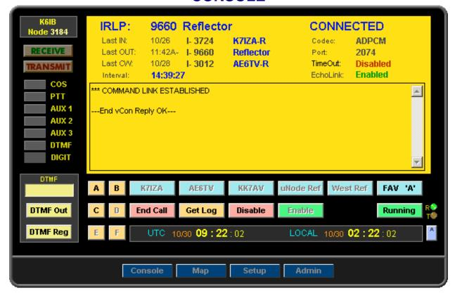
The Console Screen is the main monitor and control screen for the operation of the IRLP Node.
