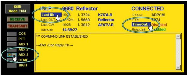
The operation of the nodes Aux outputs can be controlled by moving the mouse cursor over the desired Indicator. At that time the indicator will show a 0 and 1 box. Click the 0 to force the Output Off or click the 1 to force the Output On.
