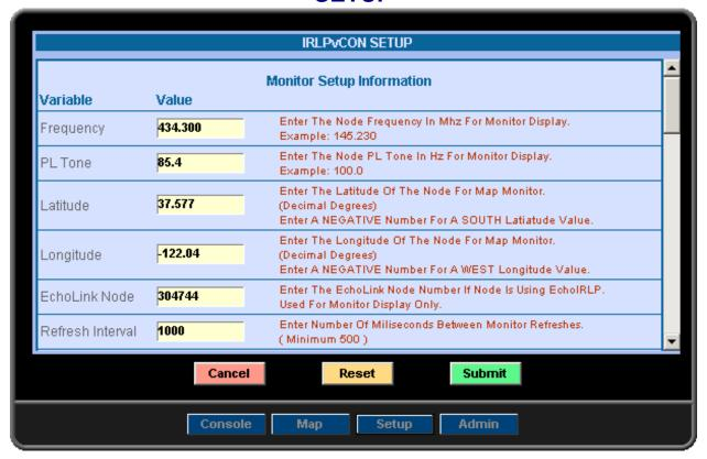
The IRLPvCON Setup Screen is used to set node information and operation variables for the operation of IRLPvCON, IRLPvMON and IRLPvMap programs. Enter the information and then click the **Submit** Button to save the information. After submitting changes it may be necessary to refresh the various monitor screens for the changes to take effect.
