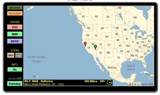
The IRLPvMAP Monitor Screen is a real-time map display that shows your node's location and the location of any IRLP node that is connected to it. To work It requires the Latitude and Longitude information be set using the Setup Screen.
