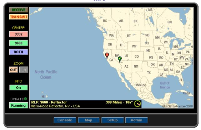
The Map Screen displays the Local location and the location of any connected IRLP node. The Local location is shown with a Red Marker. This location is taken from the Latitude and Longitude values programmed in the Setup Screen.
