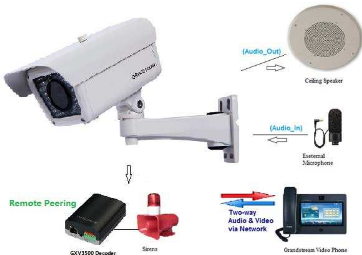
Figure 6: Application Peripheral Connection for GXV3674_HD/FHD_VF v2
