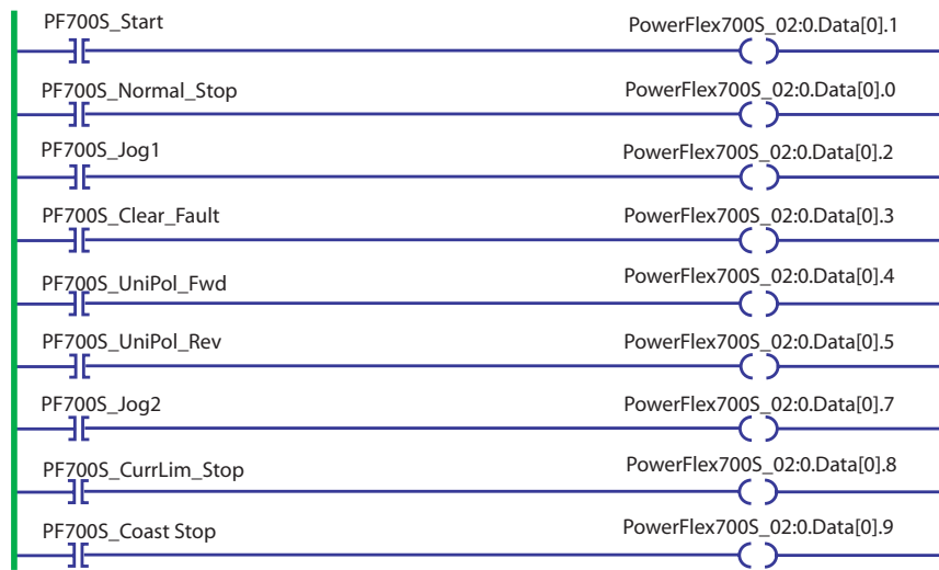
Figure 2.3 Using Bits in ControlLogix
