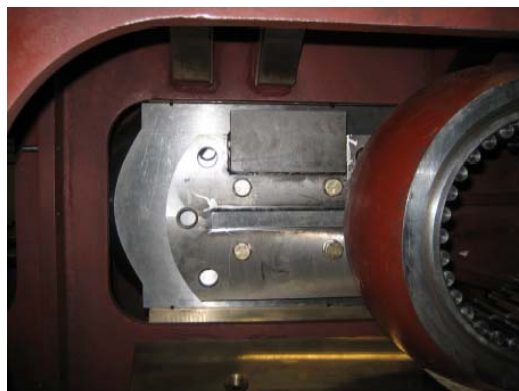
Figure 7-21 Slide Crosshead out of Guide, Remove top guide
