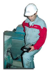
The analyser enables to measure TRUE-RMS and TRUE-PEAK values, time signal and the signal spectrum of velocity in frequency band LF and that of acceleration in frequency band LIN (vide the Technical Specification on the final page).
