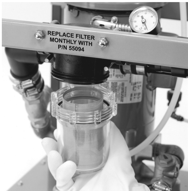
Figure 12. Intake Solids Collector Location
