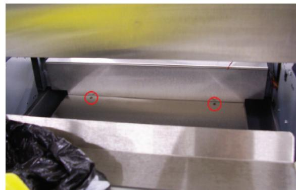
2. Next remove the four screws holding in the upper back plate.
