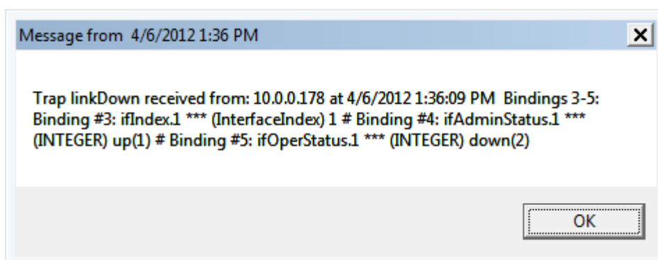
Figure 20: A pop-up message displaying some linkDown Trap notification details
