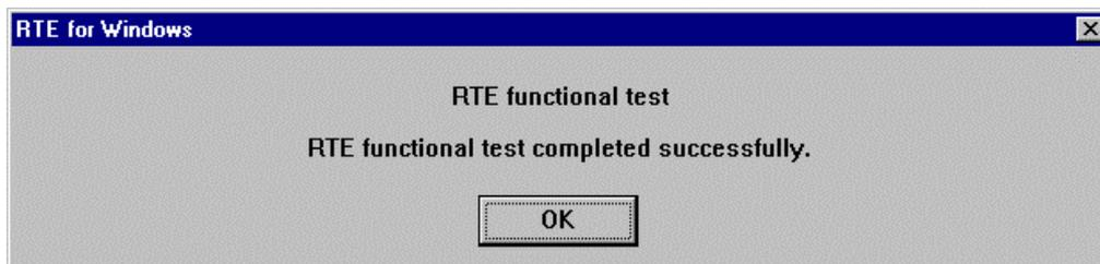
If an error occurs during the test, the user system has a failure or the JTAG/N-Wire cable is not properly connected. Check its connection.
