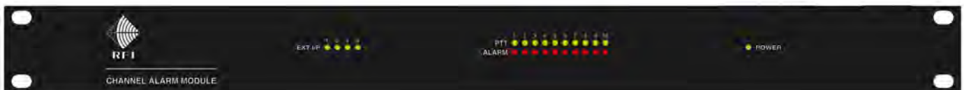
Channel Alarm Module (CAM) Front Panel Layout
