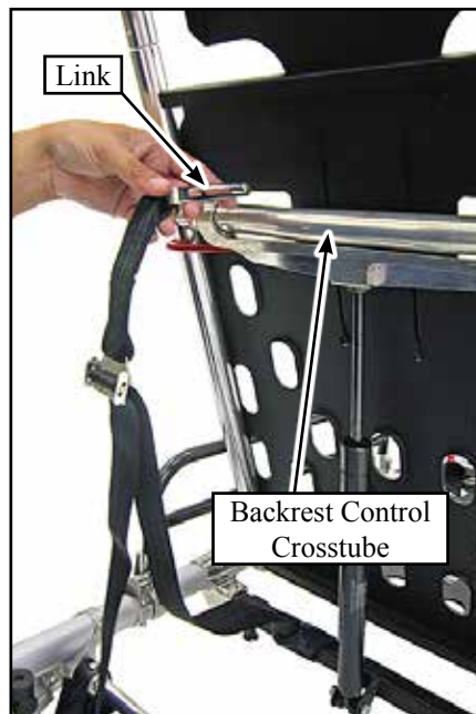
Figure 4 - Route Link Over Crosstube and Through Backrest
