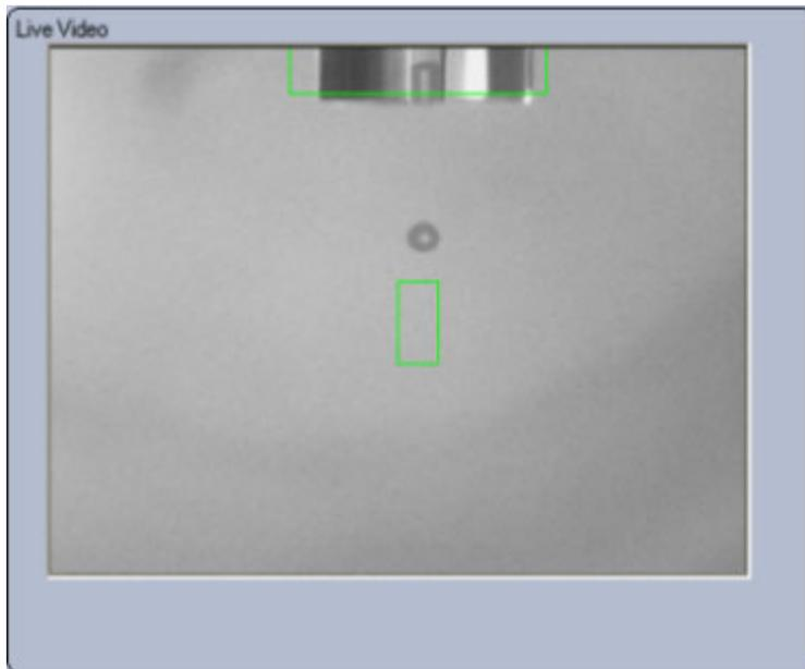
**Figure D-2. Improper Dispensing - Drop Out of Range.**
