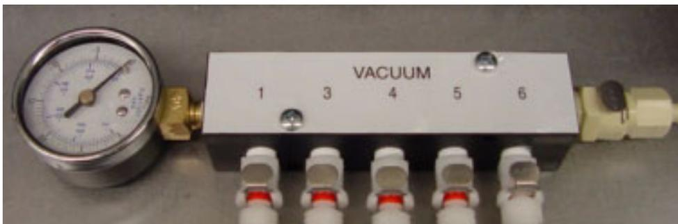
**Figure 8-1. Vacuum Manifold.**
