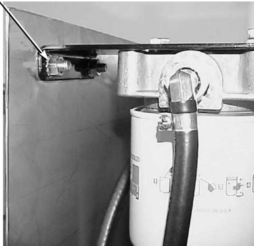
Run 12 Gauge wire from eyelet to Pin B on connector #905455 for the ground.
