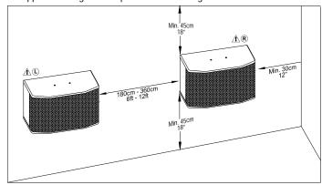
The speaker may be attached using a proprietary bracket or a pair of wall mounts screwed securely to the speaker and the wall as shown in Figure A.
