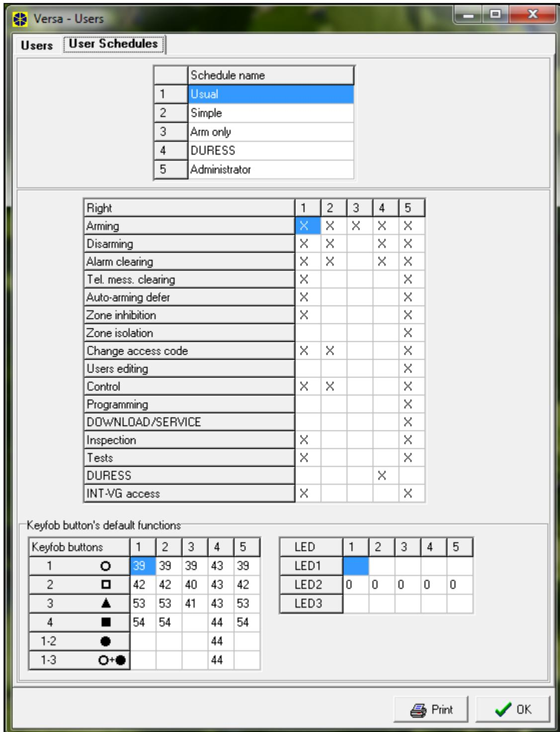
Fig. 20. Programming user schedules in the "Versa – Users" window, DLOADX program (example of settings).
