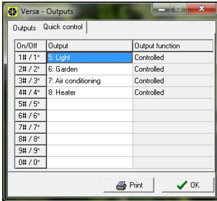
Fig. 11. Assigning the outputs to corresponding keypad keys in the DLOADX program (an example of configuration).
