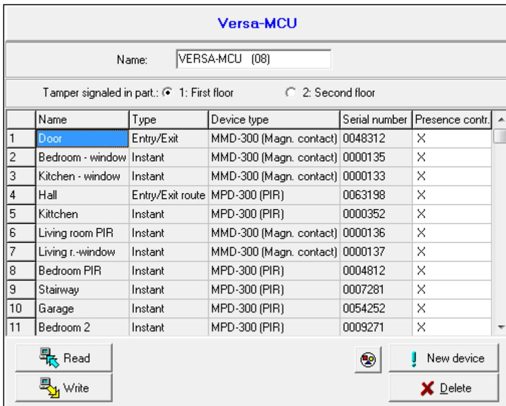
Fig. 15. Programming the settings for 433 MHz wireless system controller and 433 MHz wireless detectors in DLOADX program (an example of configuration).
