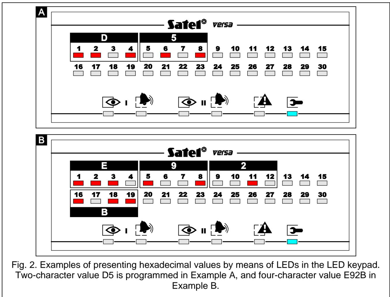
Fig. 2. Examples of presenting hexadecimal values by means of LEDs in the LED keypad. Two-character value D5 is programmed in Example A, and four-character value E92B in Example B.
