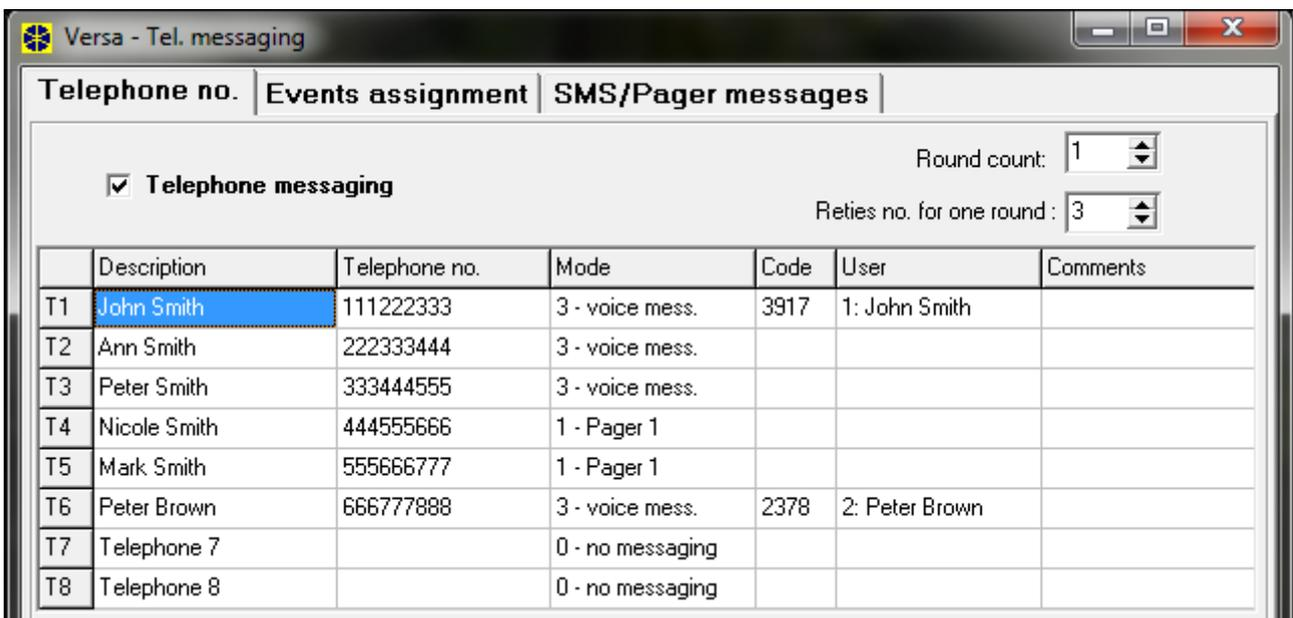
Fig. 19. Programming the messaging parameters in the DLOADX program (an example of configuration).
