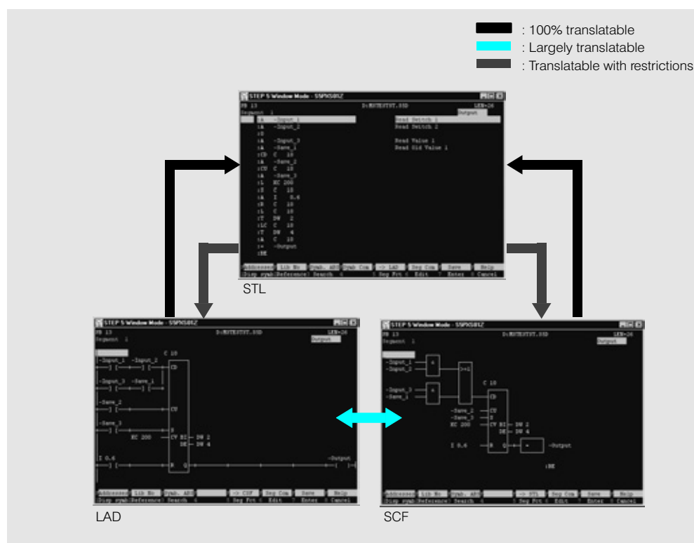
Fig. 7/3 Compatibility of the STEP 5 methods of representation
