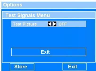
Several different test lines can be activated and deactivated. If you activate a test line you can choose the line for keying it in. The valid range for keying in the test line is between 17 – 28 and 330 – 341. Any changes have to be stored by choosing the “Store” button.
