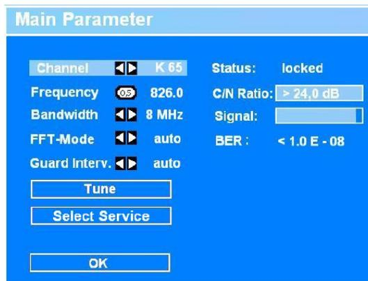
The movement between the different lines can be done with the ↑ or ↓ – keys. The parameters can be changed with the ← or → keys, or the input with the numerical keypad in the “Frequency” option.
