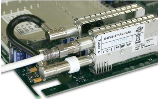
Input signal bridged from tuner A to tuner B
