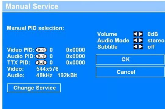
In this sub-menu, the video PID, audio PID and Teletext PID have to be entered four-digit decimal. The hexadecimal PID will be converted by the card software and displayed next to the decimal PID. If you choose a program like this and you type in wrong PIDs, there will be no error message on the OSD!
