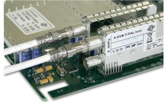
Tuner A and tuner B connected separately with input signal
