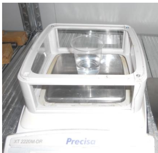
Fig. 20. Weighing a glass of water in a high precision weight scale
