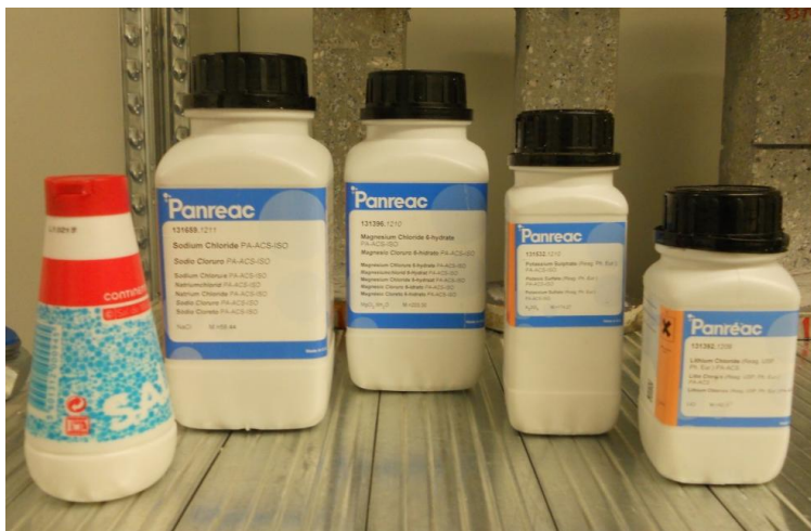
Fig. 14. Salts used for environmental control in the containers
