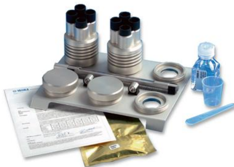
Fig. 1. Vaisala HMK 15 relative humidity calibrator
