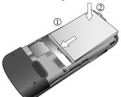
Switch off your phone before removing the battery to prevent the loss of data or settings that are not saved.
