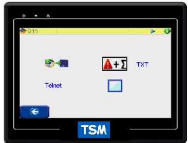
When either if these options are enabled the blender will then start logging its Alarms/batch information to the SD card or USB drive. This information can be emailed to TSM to help diagnose a problem. (The batch logging should be turned off when not in use to lengthen the life of the SD card.)
