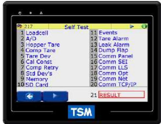
**WARNING:** The Self Test will pause the blender for 25-30 seconds and therefore should only be used when the line is stopped.
