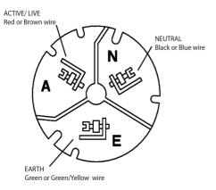
As the colours of the wires in the mains lead for the appliance may not correspond with the coloured markings identifying the terminals in your plug, proceed as follows:
