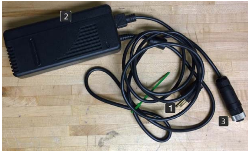
Figure 3-3: Power Supply Description
