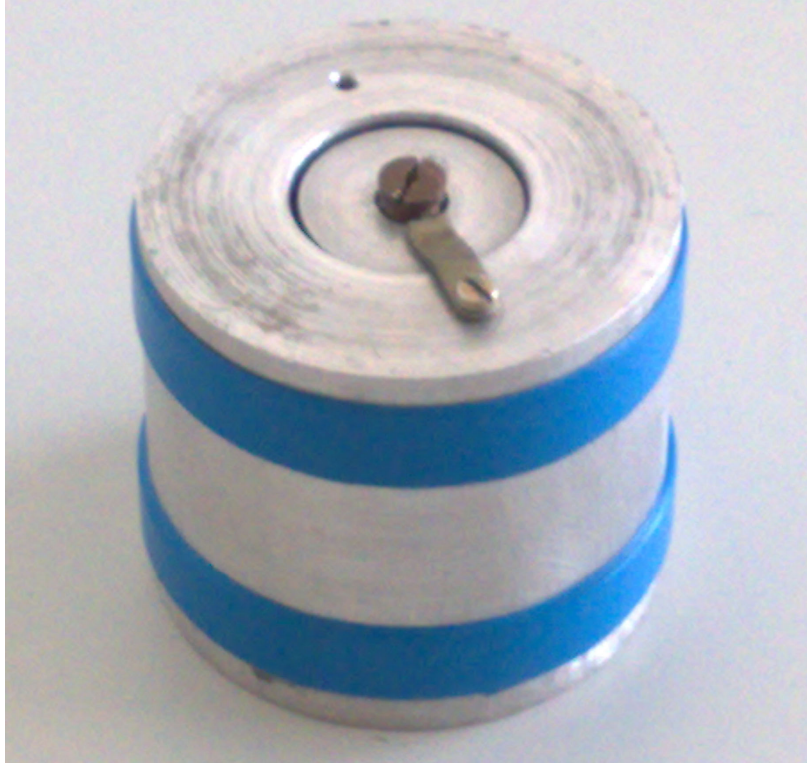
Fig. 16. Aluminum container with the beta radioactive source Sr-90 inside. Radiation is emitted through the small hole at the top (that hole has no special cover and is uncovered at all times)
