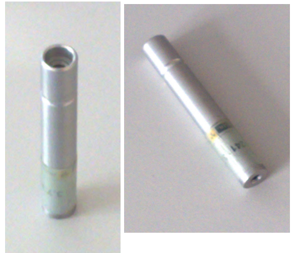
Fig. 7. The open Am-241 source (the radioactive material is at the top)
