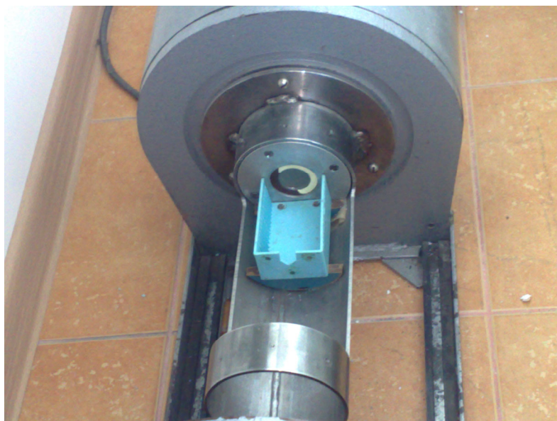
Fig. 15. The entrance window of the GM tube and the absorber holder in front of it (a slide holder is used in its place)
