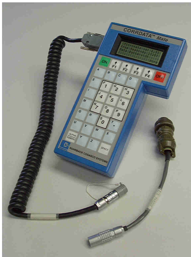
Figure 4 Corrddata Mate programmed as Micromate
