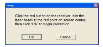
4. Following the on-screen instruction, click the red button on the receiver, aim the laser beam at the red point on screen center, and click "OK". 12 seconds later, a green dot appears on the top left corner of the projection screen.
