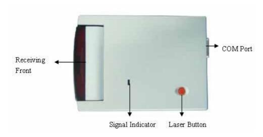
Signal indicator: When receiving infrared signal emitted by electronic pointer or light pen (or other devices), this indicator will turn green.
