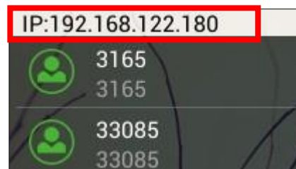
Figure 14: GXV3240 Main Screen - IP Address
