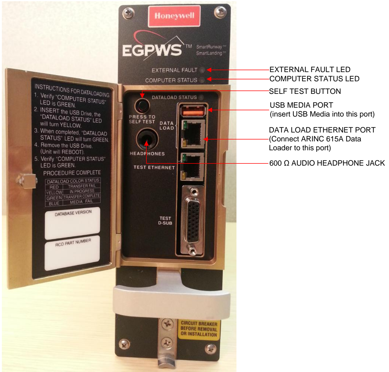
FIGURE 1: Status LEDs and USB Data load Port
