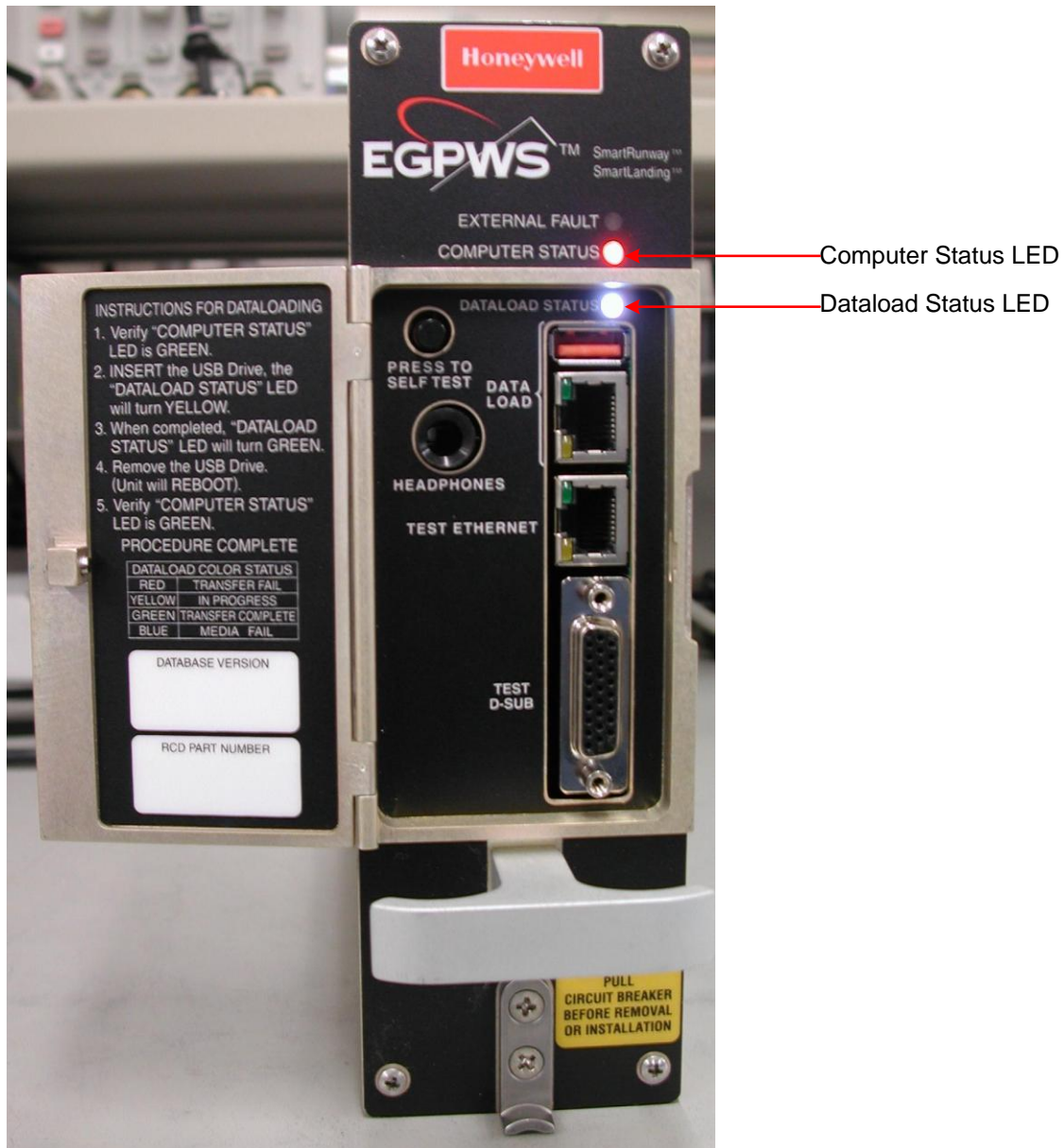
FIGURE 3: Data load Status LED
