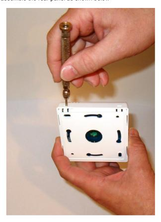
b) by the use of small screwdriver removed from the cover the PCB as shown below
