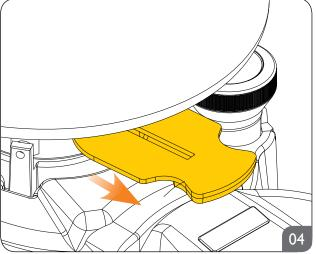
Connect the machine to the mains socket and pull the tab at the bottom of the coffee bean container to open it.
