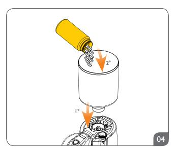
Reassemble bean hopper and fill with one cap of Grindz cleaning tablets and reopen bean stop.
