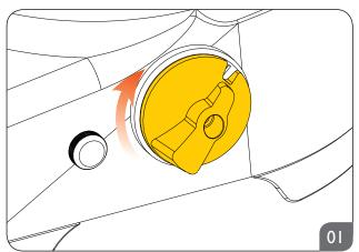
After having filled the container with coffee beans (see instructions I-4 "Starting the grinder ZENITH Manual and ZENITH On demand"), switch ON the grinder on the ON/OFF switch.
