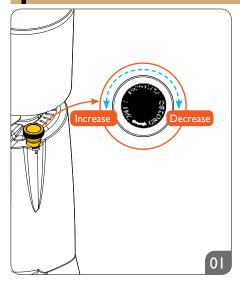
Use the grinding adjustment knob to set the grinding fineness.
