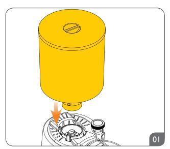
• Insert the container into its seat; positioning it so that the hole lines up with the screw on the back part of grinder.
