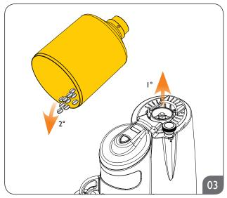
■ Turn OFF the grinder, remove the bean hopper and pour out the remaining coffee beans.
