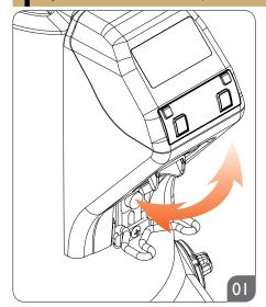
Adjust the orientation of the dispensing spout to suit the filter holder used.
