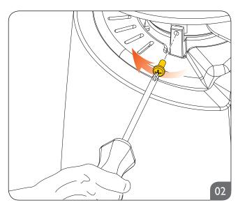
Tighten the lock screw.
