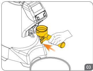
Place the filter holder onto the fork and insert it against the filter holder restraint.
