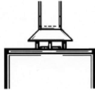
1. The vent pipe should **ALWAYS** be the same size as the outlet of the draft diverter or factory supplied vent reducer.
