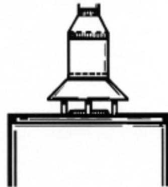
2. The diameter of a vent pipe should **NEVER** be reduced, no matter what the circumstances.
