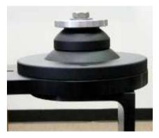
Continue gradually adding counterweights to the weight bar until the crane is just short of balanced, and then add your remote controls as the final "counterweight."
