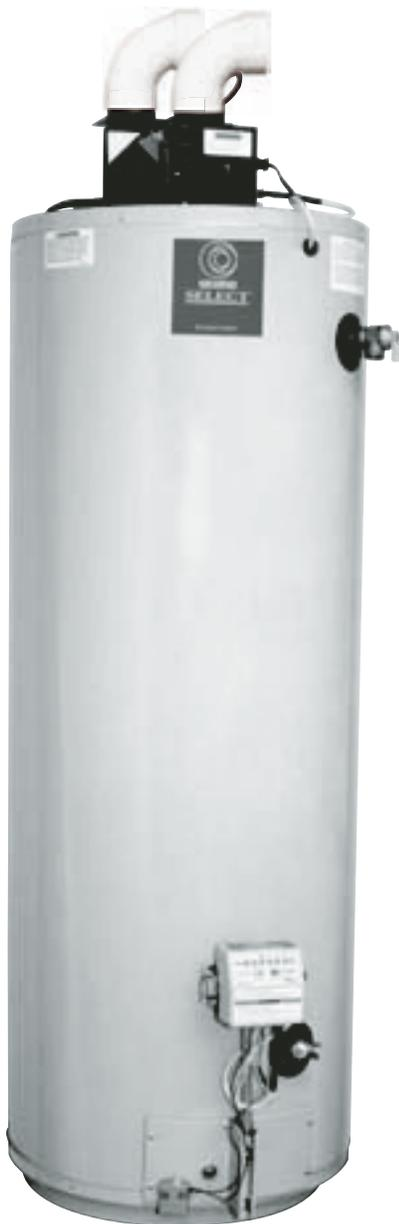
**Power Direct-Vent Design** – Two-pipe closed-combustion system draws all make-up air from outside the home, eliminating problems caused by insufficient indoor ventilation. For installation versatility, system permits combined horizontal and vertical venting and air intake runs up to 45 feet (including one 90° elbow using 3” Schedule 40 PVC, CPVC or ABS pipe).
