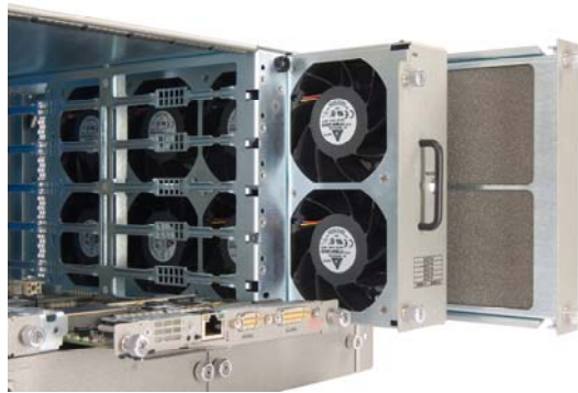
Figure 20 – Extracting a Fan Tray
