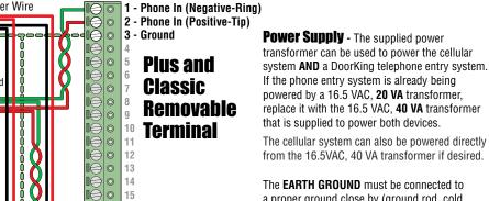
a proper ground close by (ground rod, cold water pipe in the ground, existing electrical 17 - 16.5 VAC Input Power ground (dashed lines), etc.). 18 - 16.5 VAC Input Power
