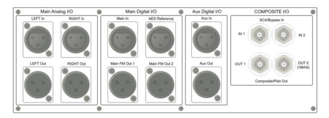
A Word about AES Reference and Sample Rates: If you need to sync the Omnia.9 to an external reference, use the AES Reference Input to ensure that the externally generated reference will be used as the main clock for the Omnia.9.
