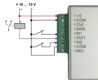
NC inputs and OC output connection diagram
