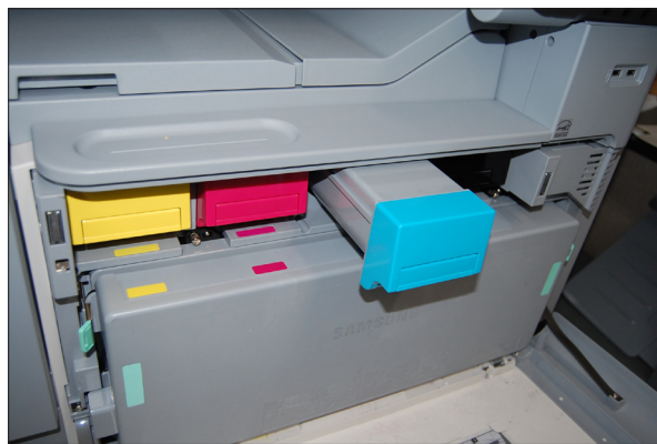
Toner cartridges simply slide into place.
