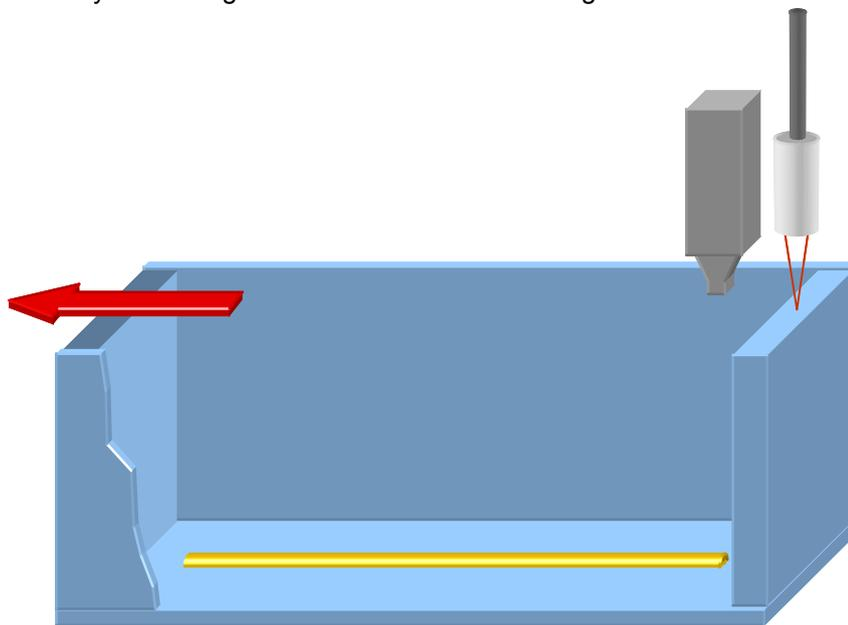
The distance between photocell and gun is 5 mm. The length of the box is 250 mm, the start delay 10 mm and the application bead length is 230 mm.
