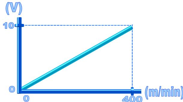
To program these values, substrates are made to pass at a low speed, e.g. 20 m/min. With the machine in movement, at this speed, enter a value in the 'Min' position on the screen, e.g. 10 Vcc and press [ENTER].
