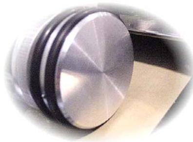
Place the encoder on smooth surface, without joints or protuberances that might make the contact wheel with the belt come out and thus 'lose' reading pulses.
