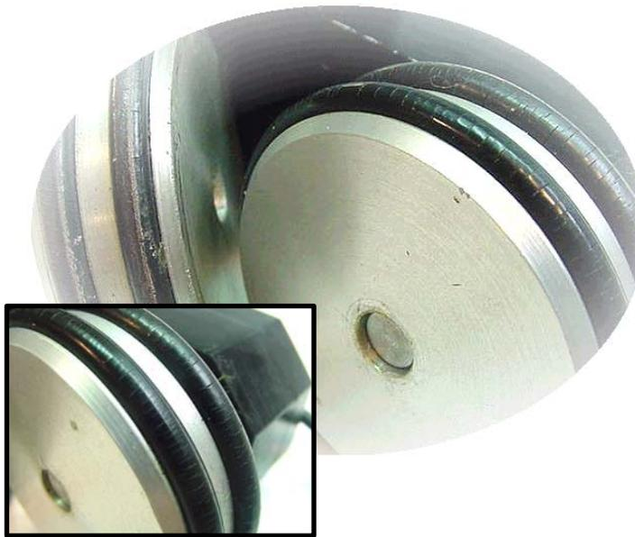
Keep the support joints of the encoder on the belt clean and in good conditions. If they are deteriorated or extremely soiled, replace them (ref. **25010016**).
