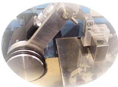
The encoder (ref. **25010007**) must be placed in a position where it can 'read' the substrate displacement speed. Avoid placing it on 'transfers' or 'pressure accumulator', belts, controlled by other motors than that of the main belt.
