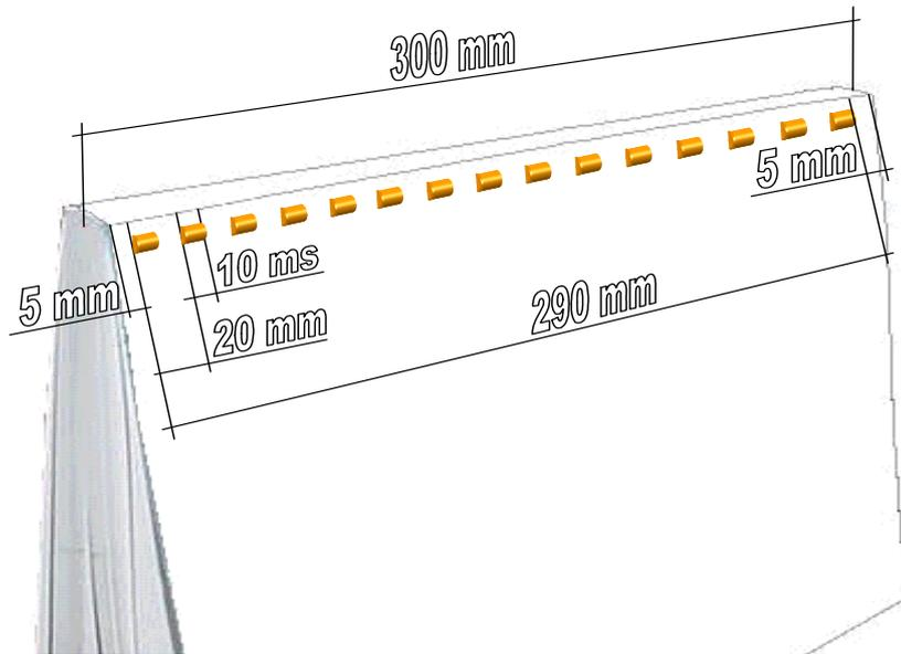
The belt speed variation belt is assumed to be irrelevant, for the purpose of the application thickness, so 0-10V signal is not used. The activation and deactivation delays compensation function will be used.
