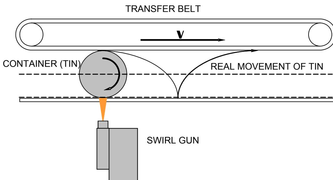
The application on the container will try to achieve, due to the characteristics of the tin used, three spiral or swirl spots, centred on the side surface.
