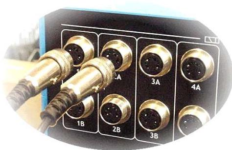
Output connection for solenoid valves (1A and 2A).
