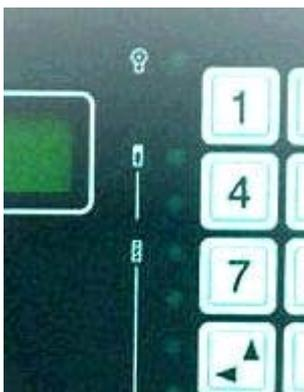
The selected output channel or channels will remain deactivated and their relative led or leds of the front panel will be off.
