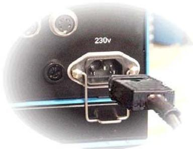
Power supply connection of the star programmer
