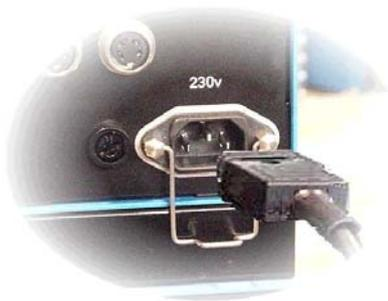
Power supply connection of the star programmer.
