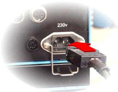
Plug the supply lead connector into the rear of the equipment.
