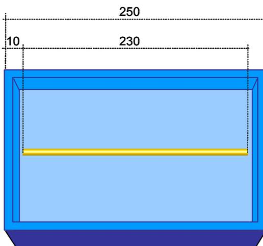
To be sure that the photocell will be cancelled when it passes over the rear edge, a value is chosen for the 'cycle security' parameter of 255 mm (length of the box – 250 mm – plus 5 mm tolerance). These 5 mm depend on the separation that exists between two boxes and can be increased if the distance between them is sufficient.
