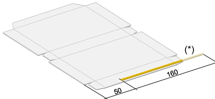
(\*) The lighter application area means that the adhesive, once it reaches the end of the box, would fall on the machine.
