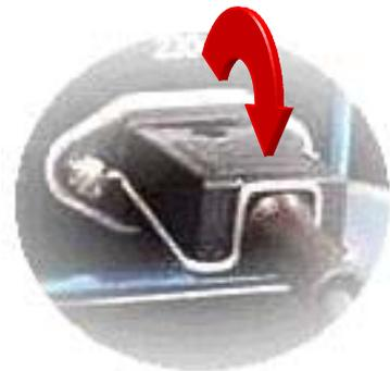
Secure connection with the flange supplied with the lead.
