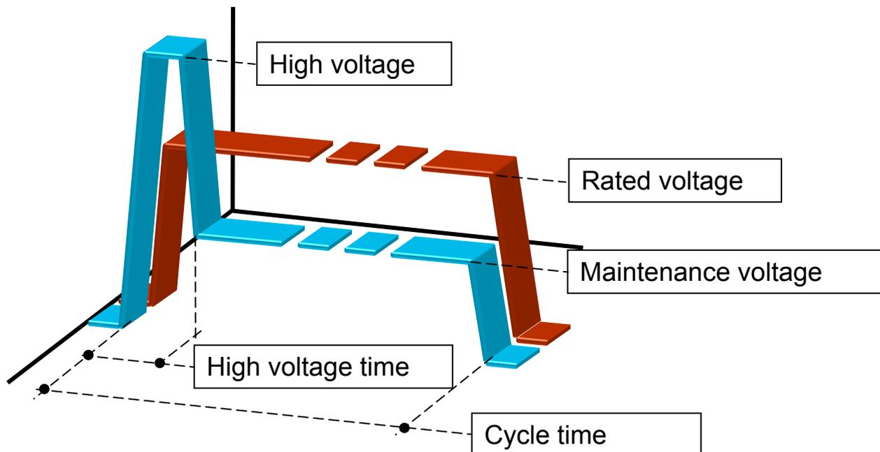
The high voltage time depends on the type of application gun used. Electric guns usually have shorter high voltage times than those ordered pneumatically by solenoid valves.
