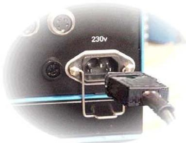
Connection of the power supply of the star programmer.
