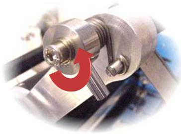
Use the tension system, by means of the torsion spring, incorporated in the belt support of the encoder (ref. **25010010**). To tighten it, gently place in the end position and turn the arm, tightening it forwards –anti-clockwise, looking from the wheel side-. Keep in this position and tighten the screw.
