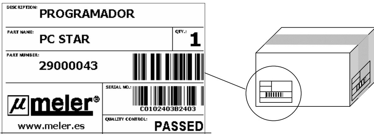
The identification ('Part number' & 'Serial n°') corresponds to the same data contained on the programmer plate.
