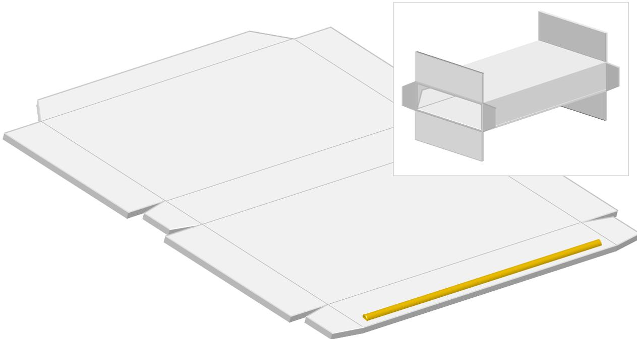
The application is simple; its difficulty lies in the fact that these cases are usually processed at high and variable machine speeds, around 120 to 150 m/min. Under these conditions, the accuracy of the application is essential and it is not possible for the bead to move due to variations in the machine speed.
