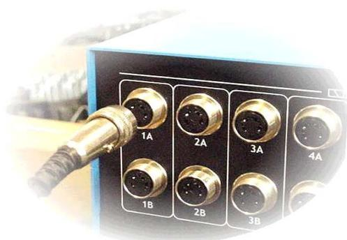
Output connection for solenoid valve (1A)
