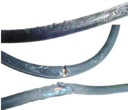
Keep the equipment power supply lead in perfect conditions. Replace it (ref. **16020001**) if any deterioration is observed.
