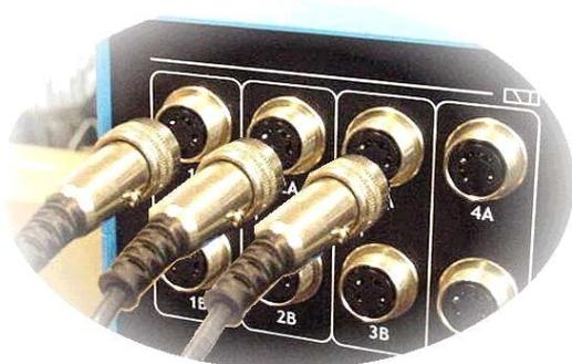
Output connection for solenoid valves (1A, 2A and 3A).
