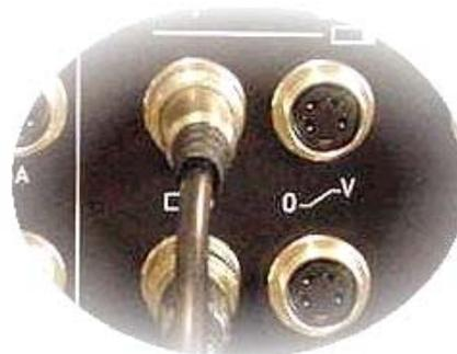
Photocell and encoder connection.
