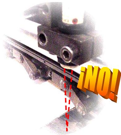
The photocells must be placed so that it detects the substrate to be glued, but, when this is not present, there must not be any reflecting surface that might activate it. The actual detection distance of each photocell must be taken into account and its activation margin respected.
