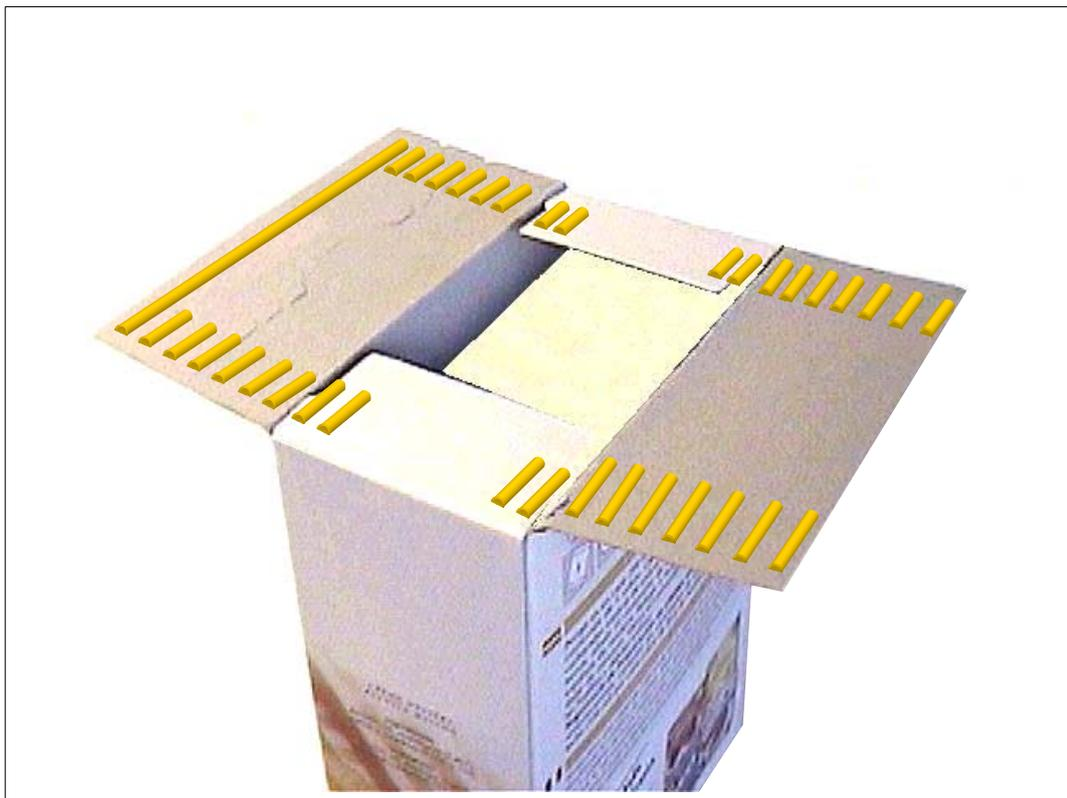
The system is comprised of two equal applications –sometimes symmetrical, depending on the layout of the injectors–, one for the lower seal of the box, before being refilled, and another for the upper seal, after dispensing the exact quantity of product. When the outer lid is finally pressed, the adhesive application creates a closed ring of adhesive, which totally isolates the product from the outside.
