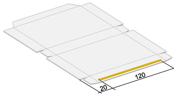
The result is now a correct start and a correct end. The compensation setting has ended and therefore, if the speed is increased to 150 m/min, the result must be the same.
