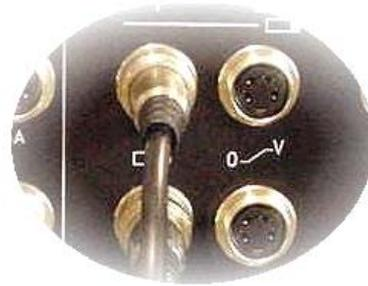
Output connection for solenoid valve (1A)
