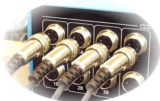
Output connectors for solenoid valves (1A, 2A, 3A, 4A).
