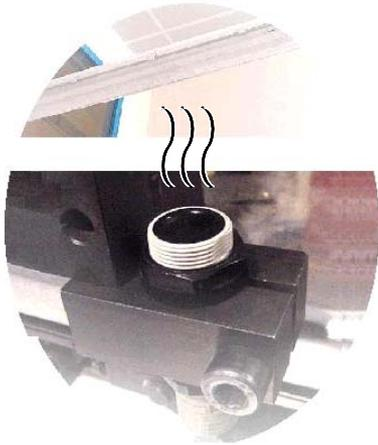
If the photocell must be placed in the opposite position –with the lens upwards– prevent any light from the main machine installation falling upon it. Although the photocells detect infrared light, some fluorescent lights might activate them accidentally.
