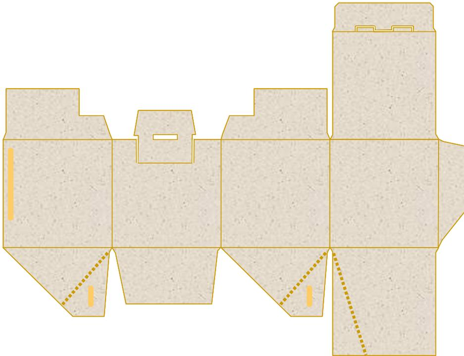
Once glued, the box is folded for later assembly, before being filled. When assembling it, press the sides from the side, the base is automatically closed.
