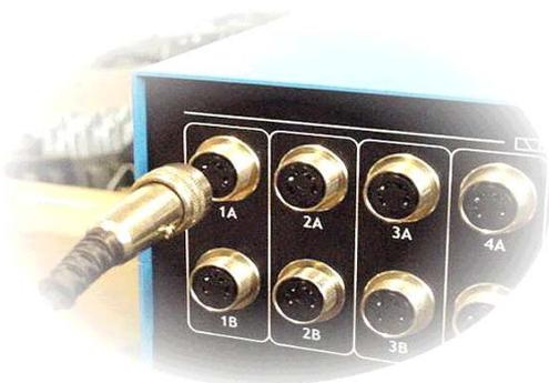
Output connection for solenoid valve (1A)
