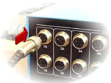
Connect the peripheral elements –guns, photocells, encoder, 0-10 V signal lead and / or gun inhibition signal lead –with the 4-pole DIN connectors.
