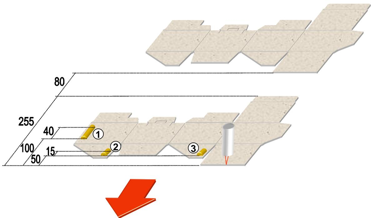
A box detection photocell connected to input '1' will be used.
