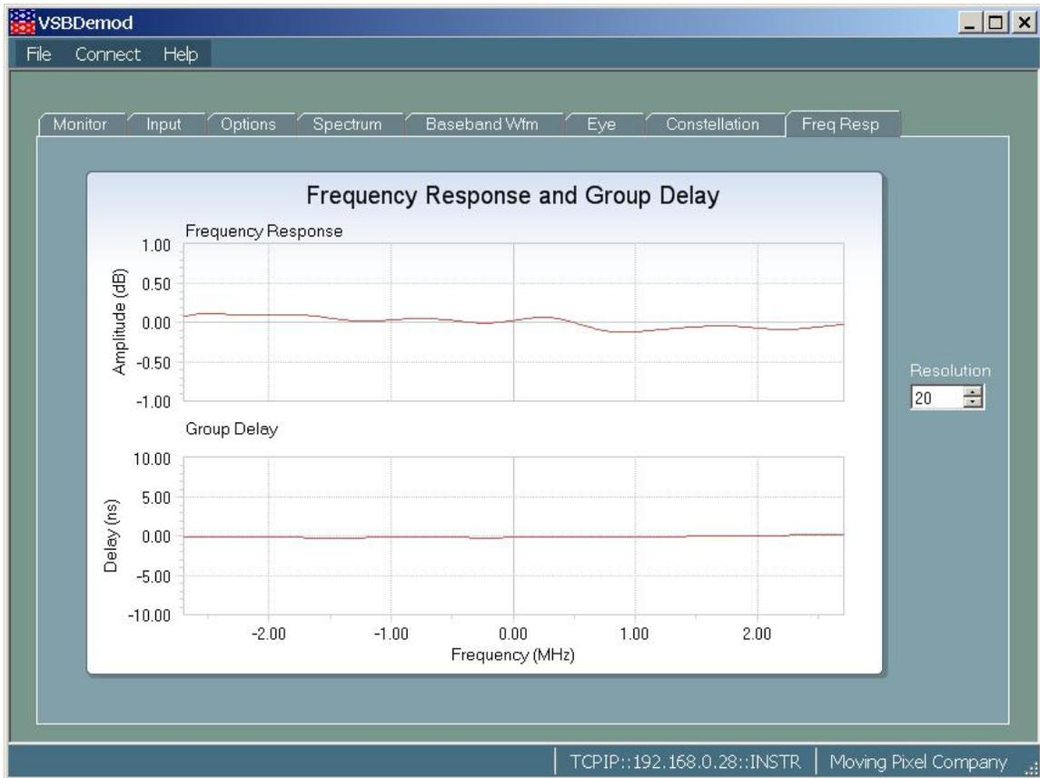
**Figure 10 – Frequency Response and Group Delay**
