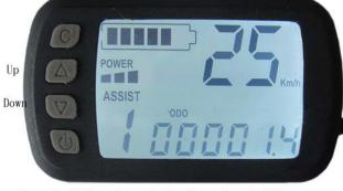
On and off/Function switch Power level Mileage
