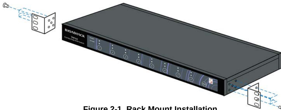
Figure 2-1. Rack Mount Installation
