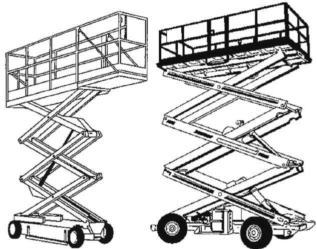
**FIGURE 1: Scissor-type Powered Platforms**
