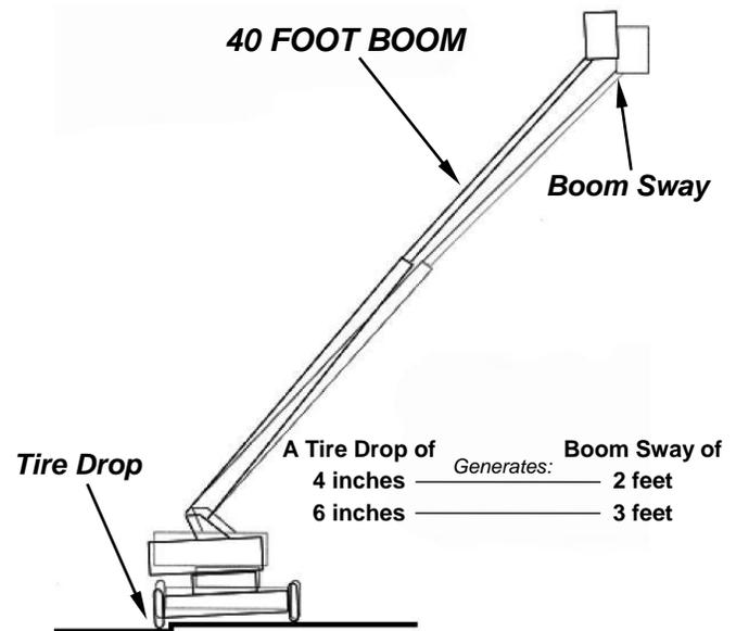
**FIGURE 10: Effect of Uneven Ground on Boom Sway**
