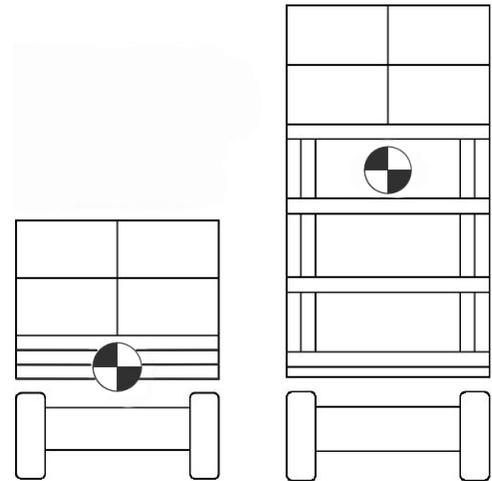
**FIGURE 8: Center of Gravity on Scissor Lifts**
