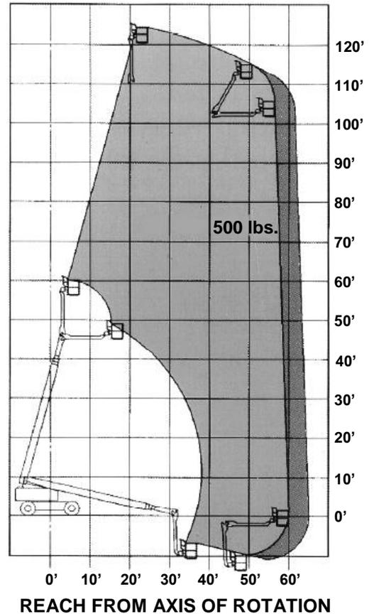
**FIGURE 6: Reach Diagram for a 36 foot Articulating Boom Platform**
