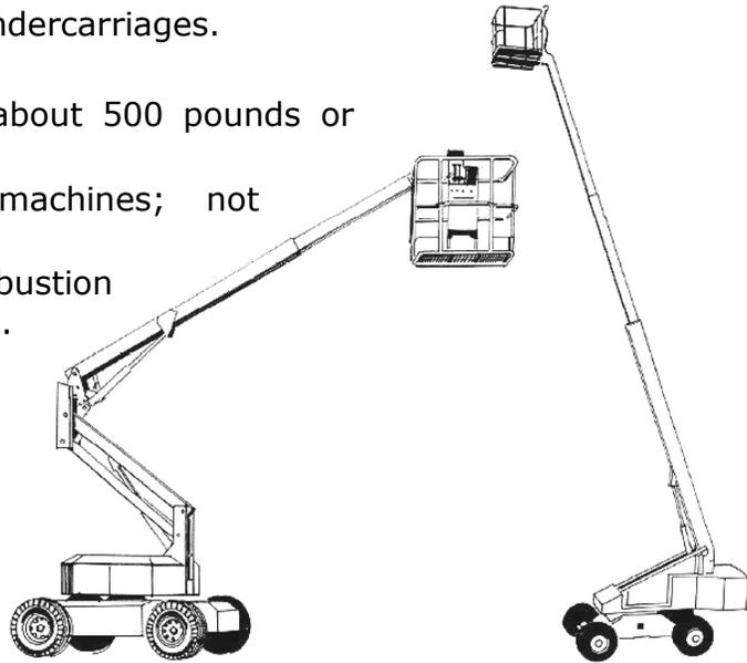
**FIGURE 3: Boom-type Powered Platforms**
