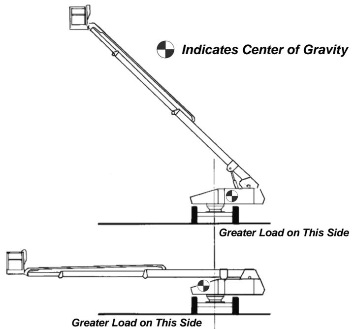
**FIGURE 9: Center of Gravity for a Boom-supported Machine**
