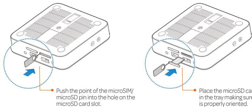
**NOTE:** The microSIM card is already installed. If you need to swap microSIM cards, the process is similar to microSD card installation.
